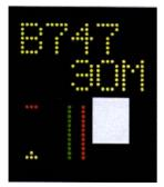
b) In this picture the aircraft is exactly 30 meters from the docking position, but is off to the right of the center line.
