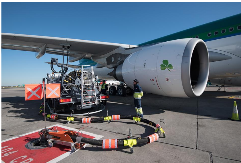
Figure 3 Safe aircraft fuelling requires training, appropriate signs and markings and detailed procedures. Dublin Airport
