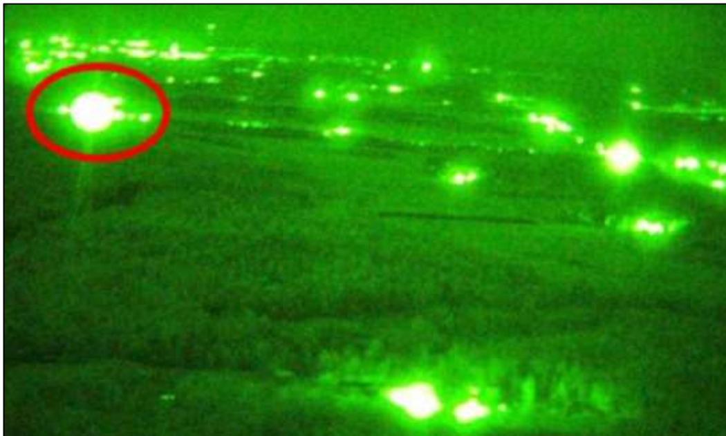
Figure 11-17. Obstruction light (circled) as seen through NVGs (source: National Research Council of Canada)
