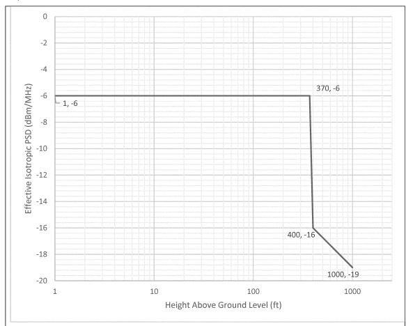
\*The notch that occurs in the curve between 370 ft AGL to 1000 ft AGL is due to the impact of the Nationwide EIRP Elevation Mask, 75 ft horizontal minimum separation distance (MSD), and 50 ft vertical MSD for a 5G tower at 350 ft AGL.
