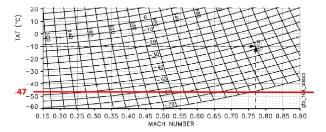
In view of forecasted OAT -71°C abeam the US East Coast, the risk of fuel freeze should be evaluated in advance. The FCOM provides general information about the development of fuel temperature during flight. The fuel temperature follows the TAT with a change rate between 3 and 12°C per hour.
